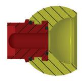
The "Quik-Change" Nozzle Tip is installed with a bayonet mount, and a simple 90° twist is all it takes to lock it into the ball. It is O-Ring sealed at the bottom and lip sealed at the top to prevent the mounting slots and tabs from becoming contaminated and difficult to disassemble.
