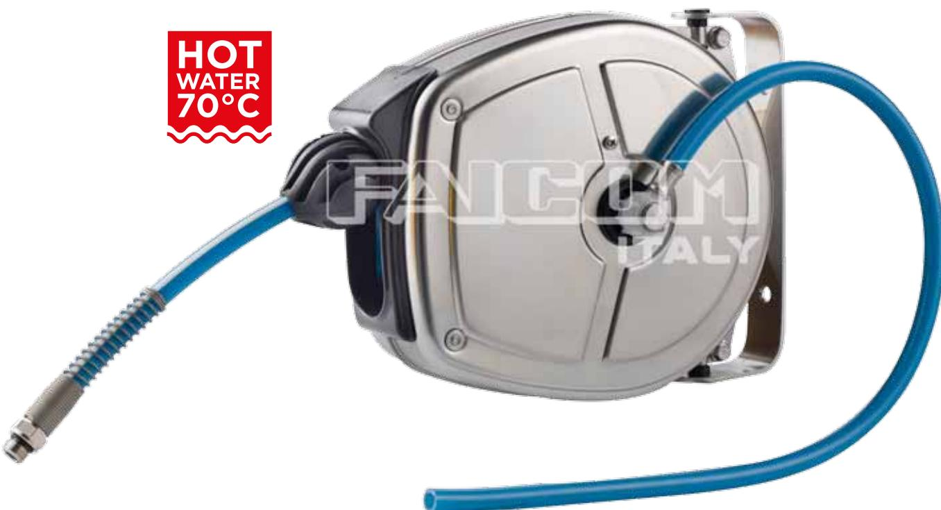
**EN** Automatic hose reels designed for washing operations with water and detergent. They are also suitable for the passage of water that comes in contact with foodstuffs and for compressed air distribution. These reels are complete with a distribution polyurethane hose reinforced with a textile braid. The connection flexible hose is 1 m long. The incorporated revolving bracket permits the orientation of the hose reels in order to follow the hose direction.
